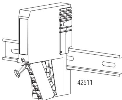
2. Remove the module to the right of the 1734-EP24DC module from its base unit.
