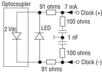
Figure 1. Sensor input
