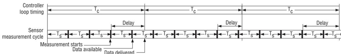
Figure 4. Asynchronous measuring mode, controller loop timing
