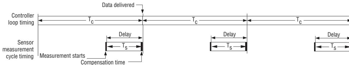
**Figure 5.** Synchronous measuring mode, Sync 1 option
