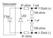
Figure 1. Sensor input
