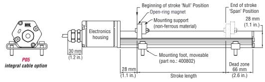
Figure 10. R-Series Model RP Profile-style sensor dimension reference (Shown with *P05* Integral cable option)
