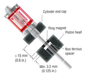
Figure 13. Model RH rod-style mounting
