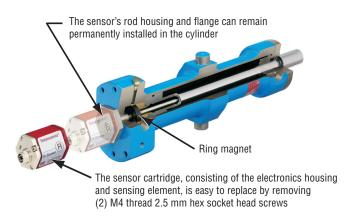
Figure 14. Fluid cylinder installation
