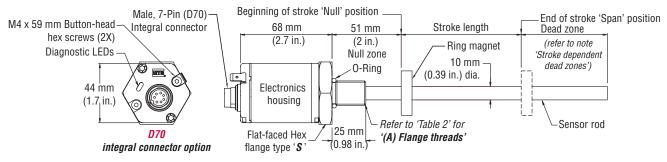
Figure 11. Model RP Profile-style sensor dimension reference (Shown with **D70** Integral connector option)
