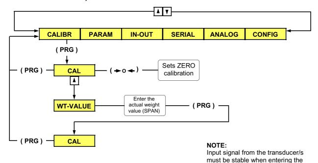
**NOTE:** Prior to calibration, the transmitter must be configured, thus giving it a set of operating parameters.
