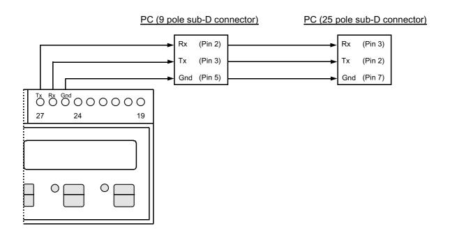
Not only the RS232, but also the RS422 or RS485 can be used for the communication with the Inovation software. Refer to Figures 3, 4, 5 depending on the desired connection.
