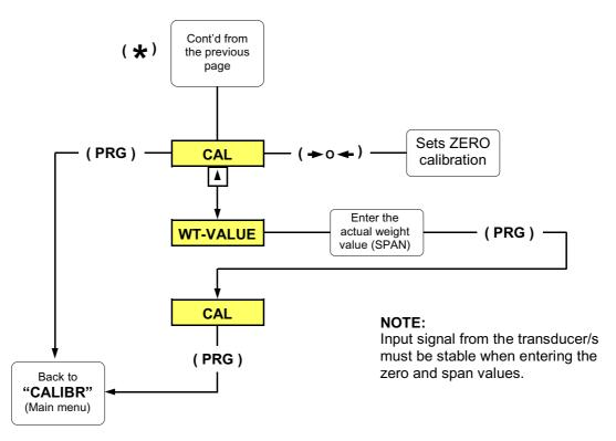
The Precise<sup>™</sup> 400 Series Transmitters can be calibrated via the front panel keys (Model 400), or with the INOVATION<sup>™</sup> configuration utility.
