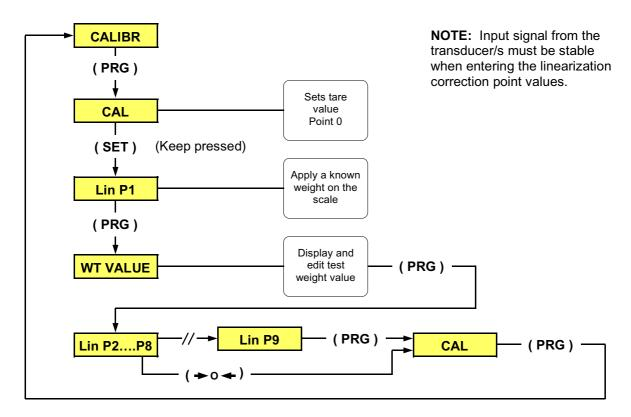
The Model 400 features a 10-point linearization option (available only with the front panel keys). Any number of points up to 10 may be used, however, the last point *must always be* the full scale value of the weighing system.
