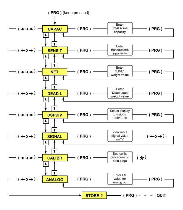
Place the unit in "Basic Configuration" mode by pressing and holding the "PRG" key until the display shows CAPAC. Use either the "UP" or "DOWN" keys to scroll through the eight basic configuration menus shown above. To set one of the following parameters, CAPAC, SENSIT, NET, DEAD L, DSPDIV, or ANALOG, press the "PRG" key to view the default or previously selected value for that parameter. To change the value, press the "O" key to select a digit,
