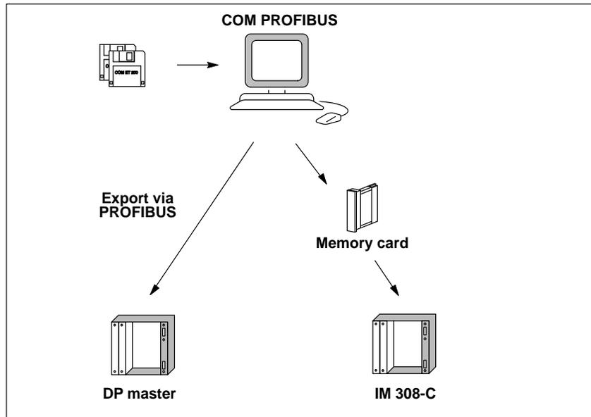
Figure 1-5 Purpose of the COM PROFIBUS parameterization software
