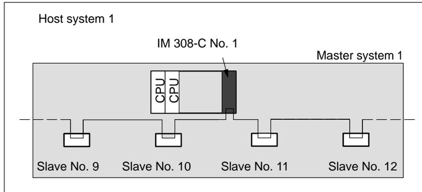
Figure 6-5 Multiprocessor mode
