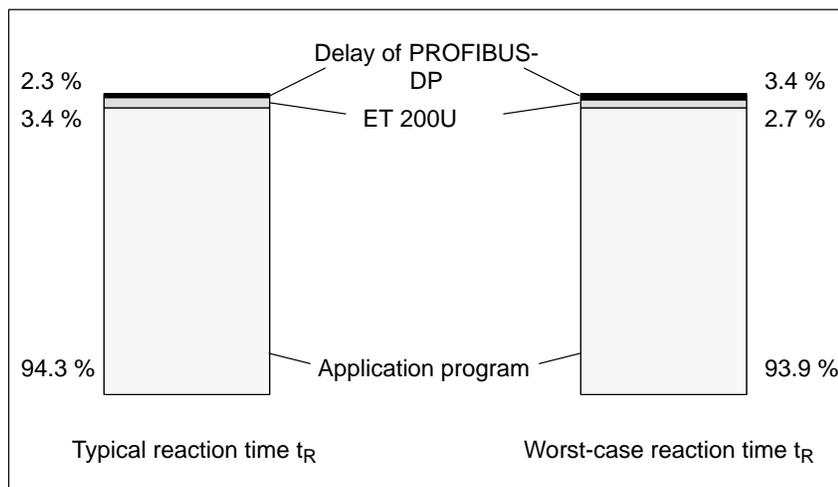
Figure C-8 Contribution of PROFIBUS-DP to the reaction time
