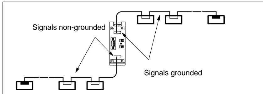
Figure 4-8 ET 200 bus segments operating as non-grounded segments
