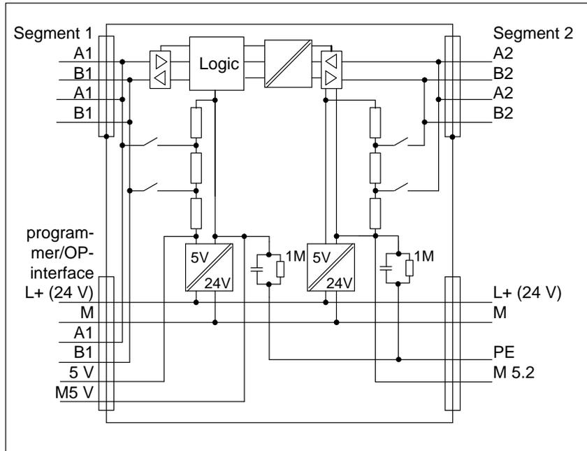
Figure 4-1 Block diagram of the RS 485 repeater
