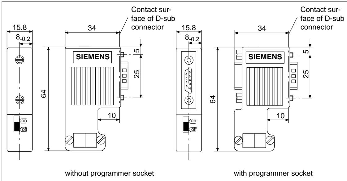
Figure E-2 IP 20 bus connector (6ES7 972-0B.11-0XA0)
