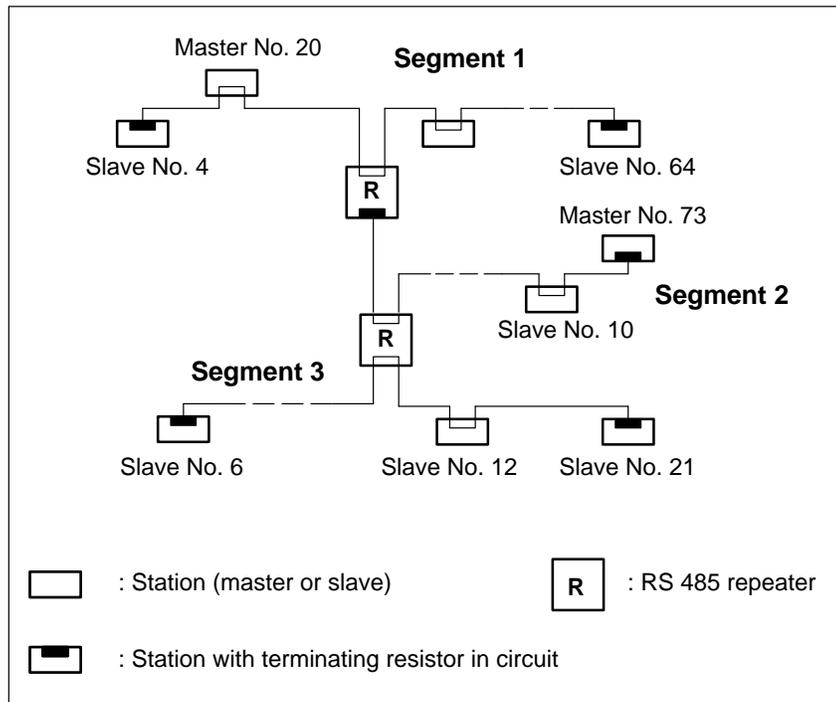
Figure 1-2 Linking bus segments with RS 485 repeaters
