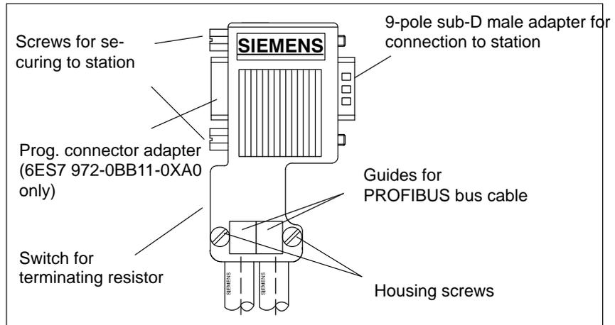
Figure 3-7 Bus connector with order number 6ES7 972-0B.11 ...
