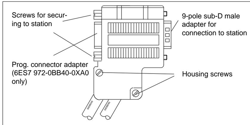
Figure 3-13 Bus connector with order number 6ES7 972-0B.40 ...
