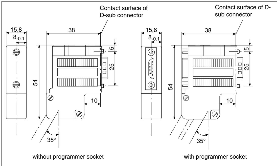
Figure E-4 IP 20 bus connector (6ES7 972-0B.40-0XA0)
