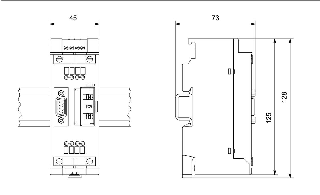
Figure E-5 RS 485 repeater on standard-section busbar
